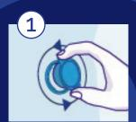
Release QRD nozzle anticlockwise and remove.
