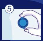
Replace QRD nozzle turning clockwise to seal.
